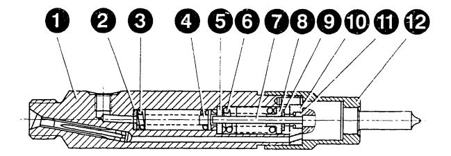
When idling, only the 1st stage of the nozzle is opened. This means that the engine runs relatively quietly at idling speed.
